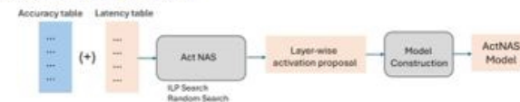
Figure 5: Combines precomputed accuracy and latency tables using Integer Linear Programming (ILP) to efficiently identify the best activation configurations.
